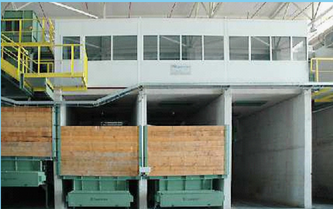
Fig.3.1.: Sorting cabins with containers for extraneous materials below
